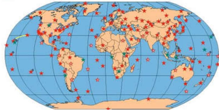
The goal of the GSN is to deploy over 128 permanent seismic recording stations uniformly over the earth's surface
